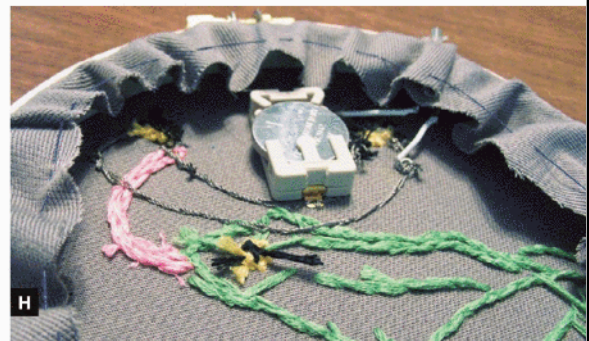
Fig. G: Sew the second switch lead to the second battery terminal. Fig. H: Gather the excess trim fabric in back with a running stitch and insert the battery.
